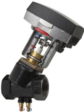
S-VARIOPULSE-VP is an electromotive, microprocessor-controlled actuator with a control signal of 0 (2) - 10 V, switchable to 3-point, with position feedback, characteristic switchable from linear to equal percentage, direction of action reversible and operation switchable to manual mode.
