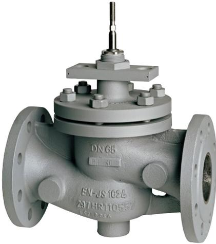
Suitable in building and process engineering for various media 0...+200 °C. Suitable with stuffing box extension or stem seal with stainless steel bellow from -10...+350 °C and for austenitic cast steel from -30...+350 °C. Suitable with stem heater for water with antifreeze compounds down to -10 °C and for austenitic cast steel down to -30 °C.
