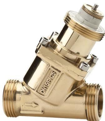
V-VARIO-DC is a pressure-independent control valve. It regulates the set volumetric flow independently of pressure fluctuations in the network. Setting independent of the valve lift for exact control over the entire input signal. The volume flow is infinitely adjustable via a fine adjustment wheel. Settings can be read from the outside. Connection M30 x 1.5 for drives of the S-KVA and VARIOPULSE-VP series.
