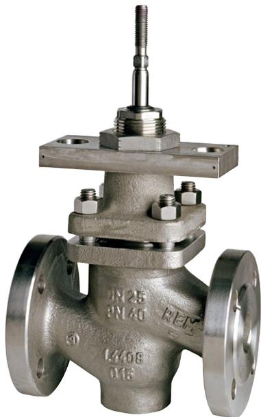
Suitable in building and process engineering for various media 0...+200 °C. Suitable with stuffing box extension or stem seal with stainless steel bellow from -10...+350 °C and for austenitic cast steel from -30...+350 °C. Suitable with stem heater for water with antifreeze compounds down to -10 °C and for austenitic cast steel down to -30 °C.
