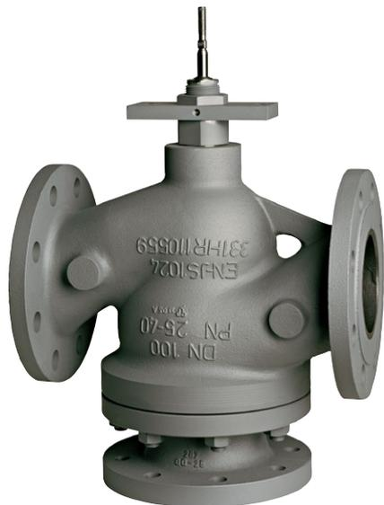
Suitable in building and process engineering for various media 0...+200 °C. Suitable with stuffing box extension or stem seal with stainless steel bellow from -10...+350 °C and for austenitic cast steel from -30...+350 °C. Suitable with stem heater for water with antifreeze compounds down to -10 °C and for austenitic cast steel down to -30 °C.
