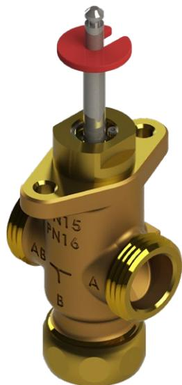
Can be used in heating, ventilation and air-conditioning systems to control the hot and cold water flow from 0...+150 °C. The valves should only be mounted in horizontal position above 130 °C. With stem heater suitable for water with antifreeze compounds down to -15 °C. The valves are tightly closed in the end positions.
