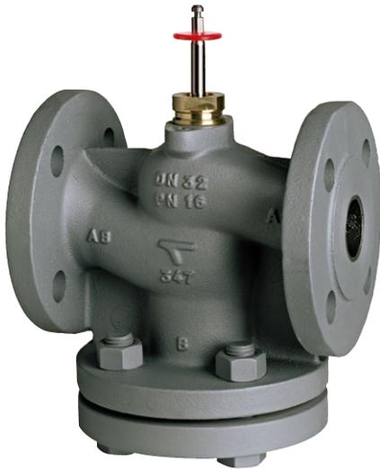
For use in heating, ventilation and air conditioning systems to control the flow of hot and cold water from 0...+150 °C. Actuator position from 130 °C only horizontal permissible. With stem heater suitable for water with anti-freeze compounds down to -10 °C. The valves are tightly closed in the end positions.
