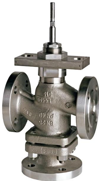
Suitable in building and process engineering for various media 0...+200 °C. Suitable with stuffing box extension or stem seal with stainless steel bellow from -10...+350 °C and for austenitic cast steel from -30...+350 °C. Suitable with stem heater for water with antifreeze compounds down to -10 °C and for austenitic cast steel down to -30 °C.
