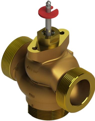
Can be used in heating, ventilation and air-conditioning systems to control the hot and cold water flow from 0...+150 °C. The valves should only be mounted in horizontal position above 130 °C. With stem heater suitable for water with antifreeze compounds down to -15 °C. The valves are tightly closed in the end positions.
