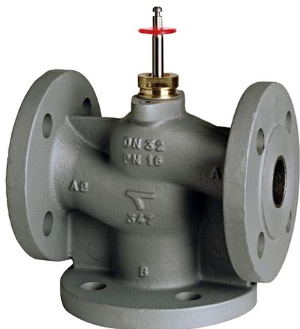
For use in heating, ventilation and air conditioning systems to control the flow of hot and cold water from 0...+150 °C. Actuator position from 130 °C only horizontal permissible. With stem heater suitable for water with anti-freeze compounds down to -10 °C. The valves are tightly closed in the end positions.
